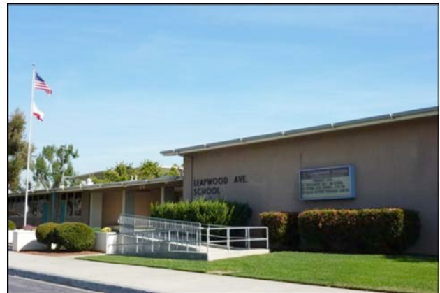
Figures 48. and 49. If ADA-compliant access cannot be accommodated at primary entrance without damage to character-defining features, consider using the California Historical Building Code and its alternatives for ADA-compliant access on secondary entrances. Install ADA-accessible ramps in a way that allows for ease of access while also limiting visual obstruction of important character-defining spaces and features to the maximum extent feasible. Source: LAUSD, 2014.
